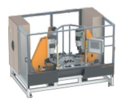
Riveting center (X, Y, Z), multi-riveting with 3 CNC units.
